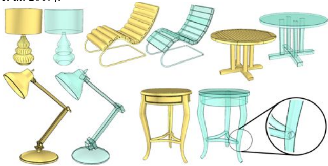
Figure 15: Controllers (shown in cyan), either a cuboid or a generalized cylinder [Zheng et al. 2011], serve as high-level deformation handles for structure-aware deformation of man-made shapes [Xu et al. 2011]. The numbers indicate the number of controllers needed, showing that a small number of controllers usually suffice for the modeling tasks.
