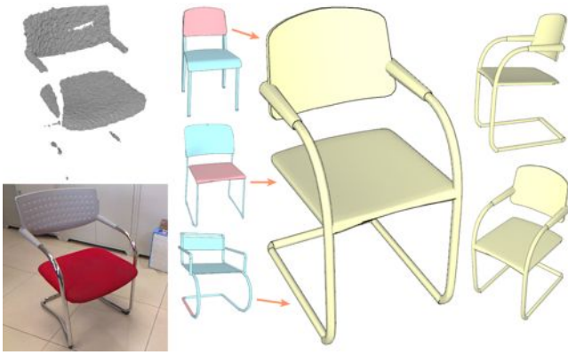
Figure 27: Structure-aware 3D model reconstruction from Kinect data. The reconstruction is based on retrieving and then assembling parts taken from multiple example shapes in a small shape repository, while preserving the built-in structures of the examples [Shen et al. 2012].
